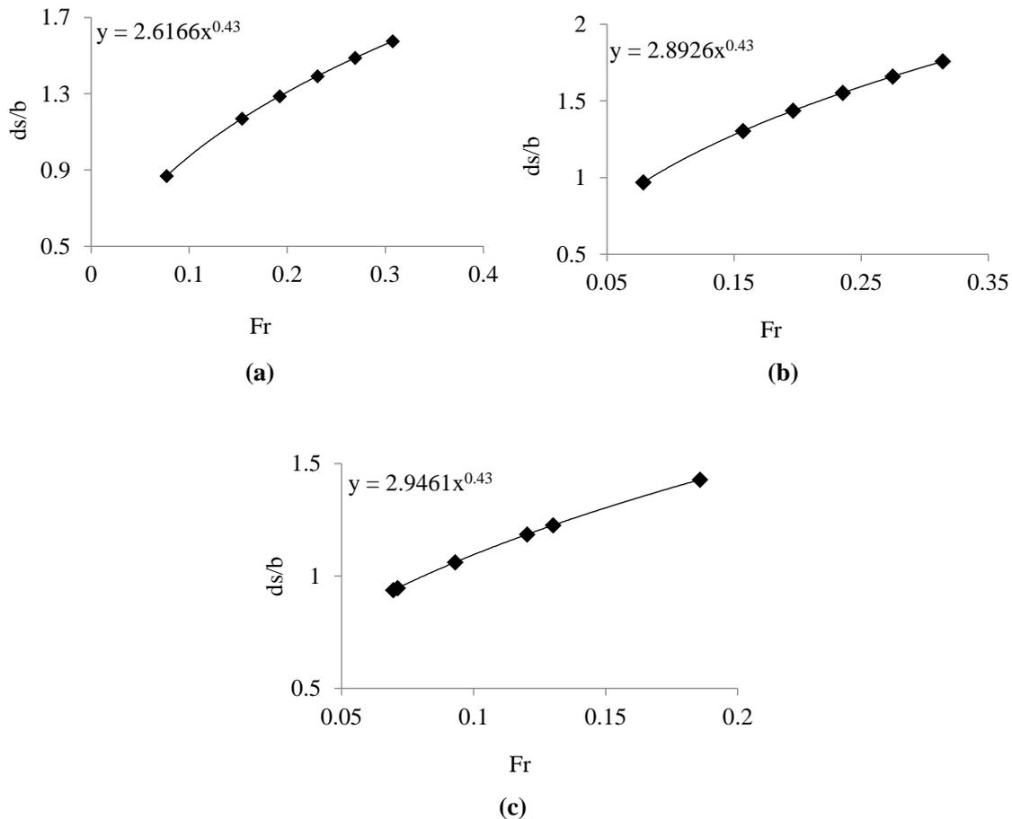
Figure 13: Variation of scouring with Froude number in (a) Machmara , (b) Burima and (c) Subhas Bridge
