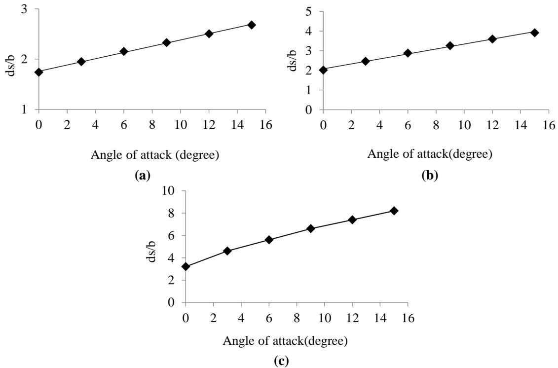
Figure 14: Variation of scouring with the angle of attack in (a) Machmara, (b) Burima and (c) Subhas Bridge
