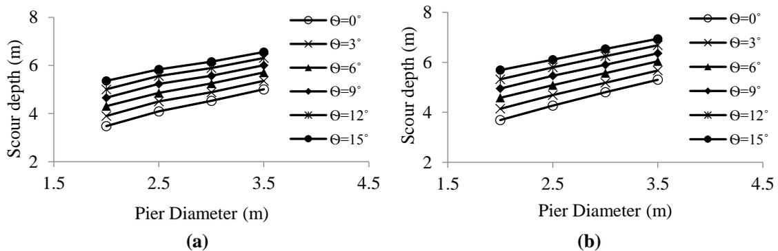
**Figure 6: Variation in scour depth with pier diameter for different angles of attack for Machmara bridge (a) full waterway and (b) Restricted waterway**
