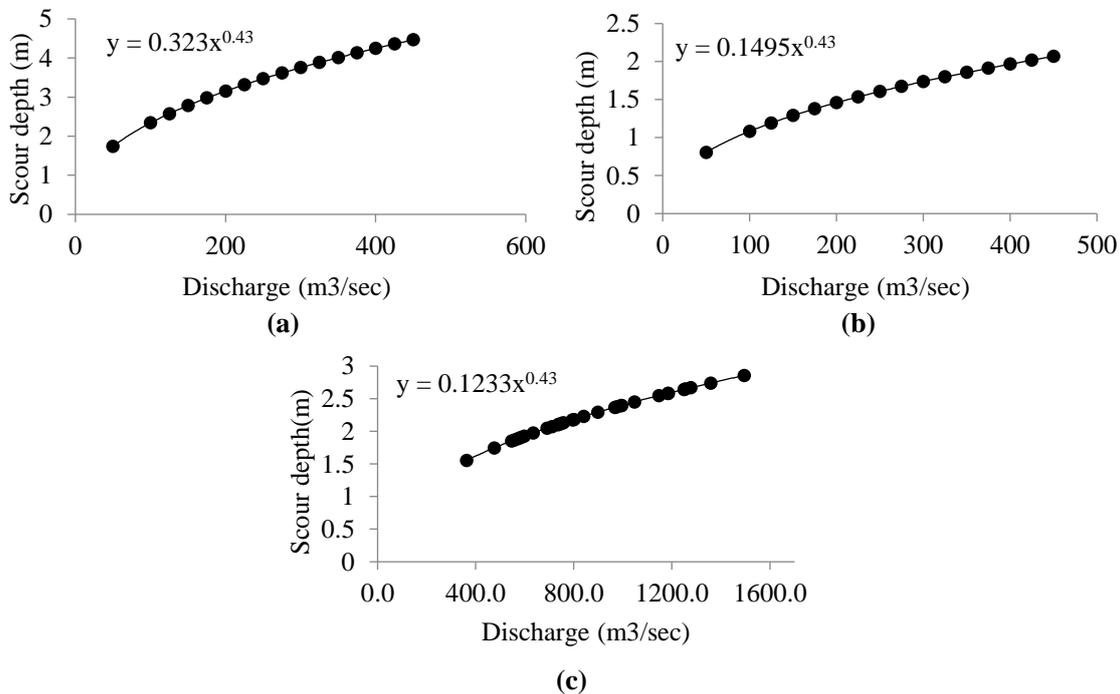
Figure 11: Variation of scouring with discharge in (a) Machmara, (b) Burima and (c) Subhas Bridge
