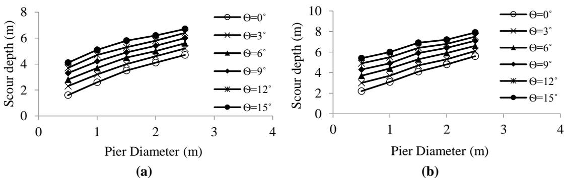
**Figure 8: Variation in scour depth with pier diameter for different angles of attack for Subhas Bridge (a) full waterway and (b) Restricted waterway**
