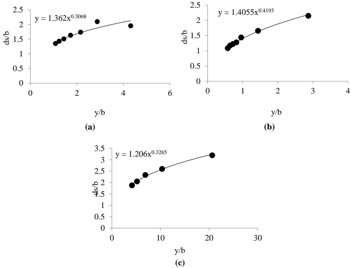
Figure 12: Variation of scouring with flow depth in (a) Machmara, (b) Burima and (c) Subhas Bridge
