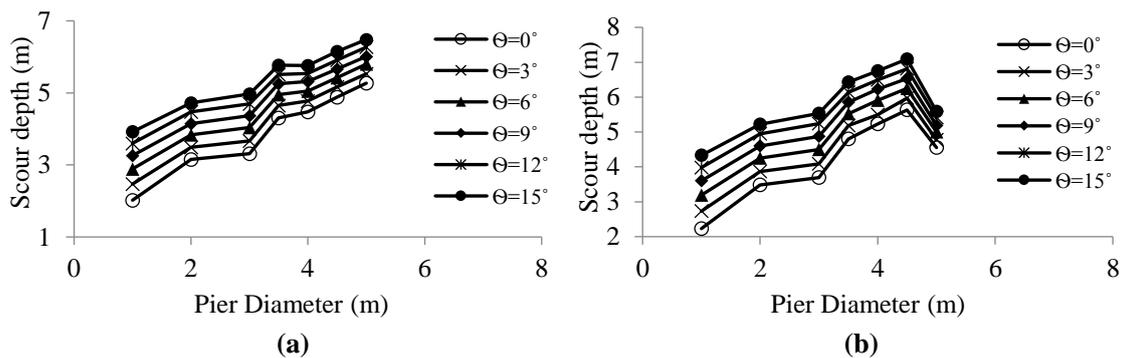
**Figure 7: Variation in scour depth with pier diameter for different angles of attack for Burima Bridge (a) full waterway and (b) Restricted waterway**
