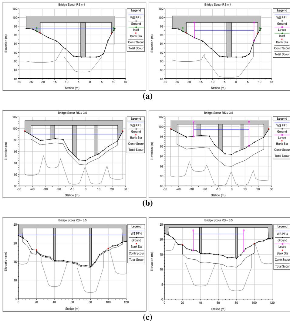
Figure 9: Scour depth using HEC-RAS tool in (a) Machmara, (b) Burima and (c) Subhas Bridge Sight
