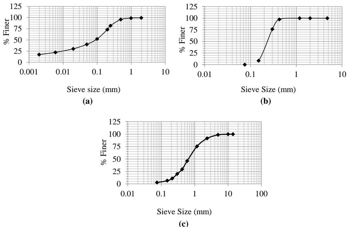
Figure 5: Particle size distribution for the sediment sample of (a) Machmara Bridge, (b) Burima Bridge and (c) Subhas Bridge
