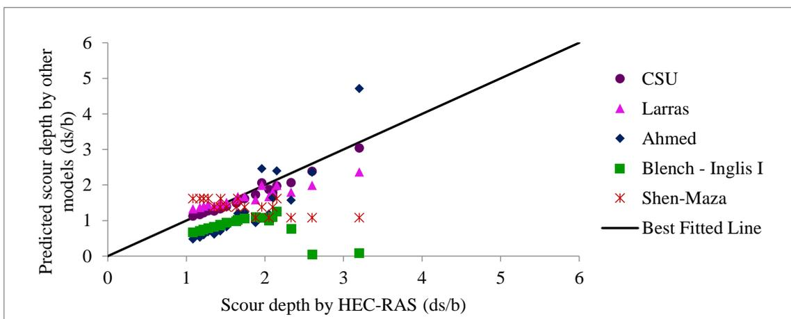
Figure 10: Comparison of predicted scour depth between the HEC-RAS model and other empirical models
