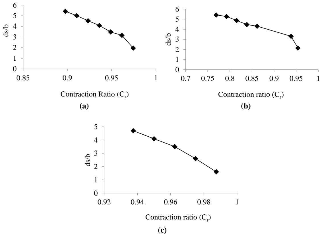
Figure 15: Variation of scouring with contraction ratio in (a) Machmara, (b) Burima and (c) Subhas Bridge
