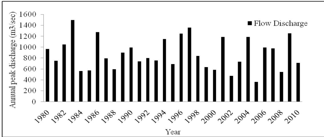
Figure 1: Peak discharge data of Gomati River for the period 1980 – 2010
